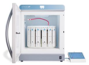
Hot block digestions suffer from long digestions, airborne contamination, poor digestion quality, and poor recovery of volatile compounds. Closed vessel microwave digestion has proven to be an effective technique with fast, complete digestions, clean environment, and full recovery of volatile compounds.
