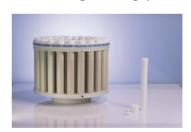
The MAXI-44 is a high throughput rotor capable to digest a large variety of food samples, improving the throughput in the labs.
